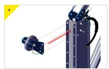
Present the sheave bracket to the top of the column.
