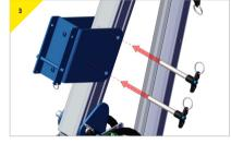
> Insert the pins provided with the bracket.
