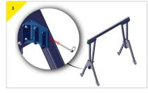
> Prepare the bracket to receive the device, and remove the pin supplied with the bracket.
