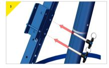
> Insert the pins provided through the bracket.
