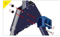
Present the bracket to the trap plate, insert and secure the top and bottom M12 bolts supplied with the bracket.
