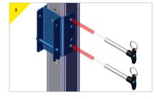
> Insert pins provided to secure bracket to section.
