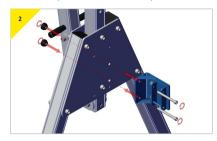
Present the bracket to the trap plate, use the centre holes in the trap plate, insert and secure the M12 bolt supplied with the bracket.
