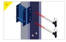
Insert the pins provided to secure bracket to the section.
