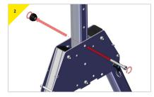
> Remove the top bolt from the trap plate.
