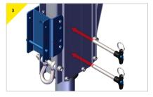
Insert the pins provided with the bracket.
