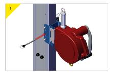
Insert the pin provided with the device to secure the block to the bracket.
